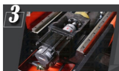
Gernardy Brand Reduction Gear Installed on Y axis, it can protect the ball screw transmission and keep the smooth operation of the mechanism.
